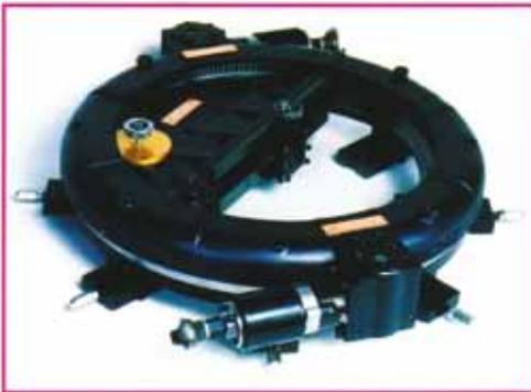
The Silk AX0244 flange facing and grooving machine is constructed from the highest quality materials. It is designed to give machine shop accuracy combined with portability and ease of handling for work on flanges from 0"-23" diameter. The machine consists of three modules:
