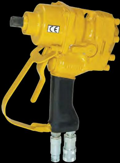
This **Underwater Impact Wrench** is the Stanley IW12 is a 3/4" square drive tool with adjustable impact intensity from 250-1200ft.lb. (340-1632Nm). Stanley Impact Wrenches can be operated over wide flow ranges, in the case of the IW12, 15-45lpm. The IW1234001 Model comes complete with quick disconnect couplers.
